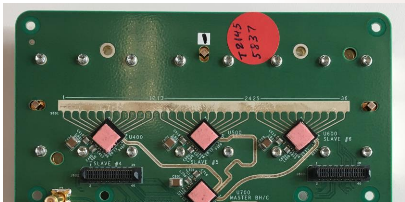
Back: RFICs connecting to antenna feeds
