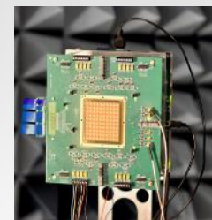
28GHz phased-array ICs and phased-array antenna modules (PAAM)
