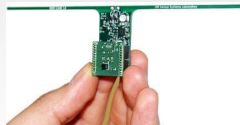
The WISPCam (Wireless Identification and Sensing Platform Camera) tag.
