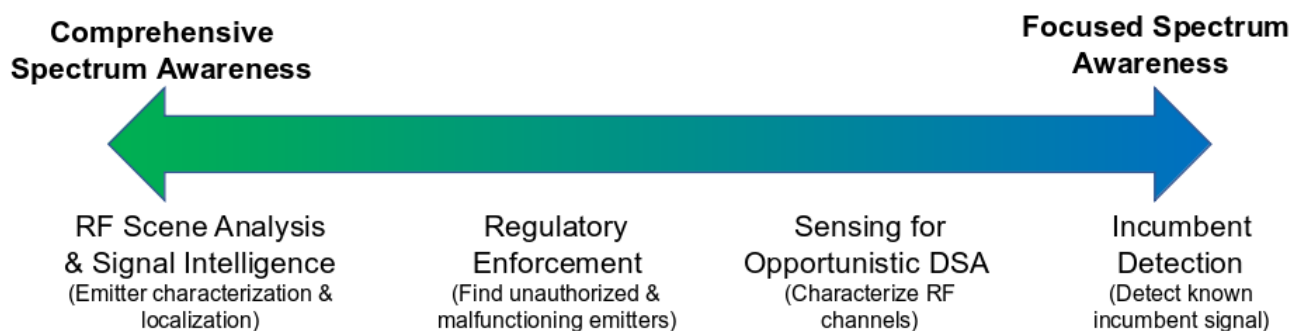
Figure 22: Continuum of Spectrum Awareness Use Cases Based on RF ML Model Inferencing and Prediction Capabilities
