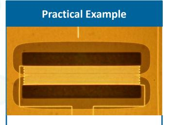
Humidity, temperature, corrosion, gas and gas flow velocity sensors, monolithically integrated in a 3 x 3 mm<sup>2</sup> chip
