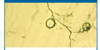
Self-healing materials able to recover from cracking and treeing due to high electrostatic stress
